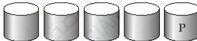
(e) RAID 4: block-interleaved parity
