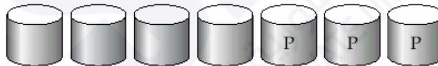
(c) RAID 2: memory-style error-correcting codes
