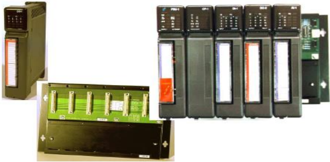
Figure (3.2) PLC Hardware
