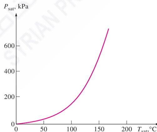
drops by a little over 3°C. Note that the atmospheric pressure at a location, and thus the boiling temperature, changes slightly with the weather conditions. But the corresponding change in the boiling temperature is no more than about 1°C.
