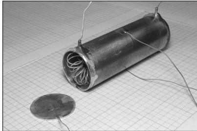
Use actual data from the experiment shown here to obtain the **latent heat of fusion** of water. See end-of-chapter problem 3–146.
