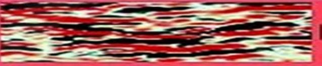
A seismic reflection example showing reflections that are wavy and somewhat fragmented, but still show some degree of continuity. The background is red.                   |
