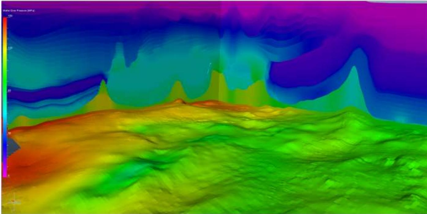
*3D Pressure computation. Through its robust and rigorous simulator, TemisFlow accounts for water flow, compaction tectonic loading, chemical compaction, deagenetic seals and shale dehydration, hydrocarbon buoyancy, hydrocarbon source, hydraulic fracturing*
