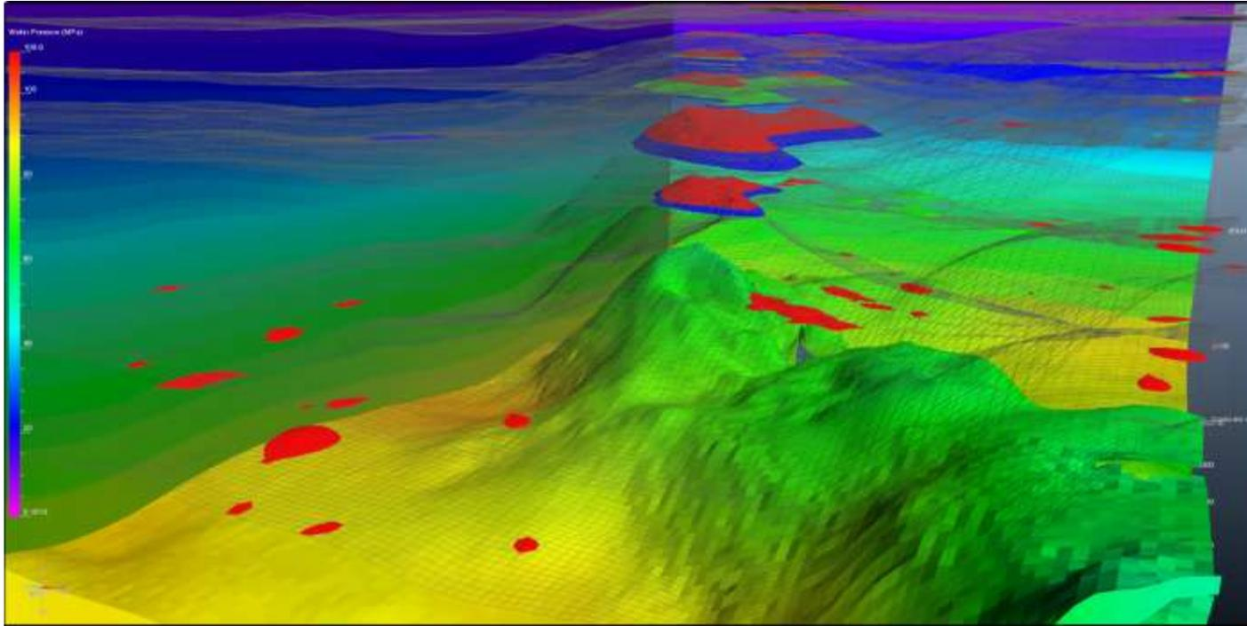
*Trap Charge Assessment: oil and gas accumulations in several reservoirs, pressure field in background.*
