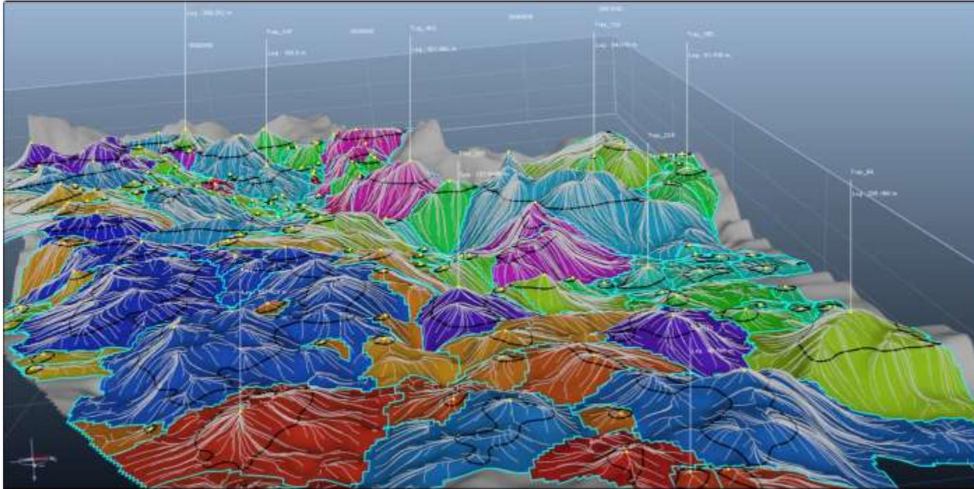
*Structural map drainage area and trap analysis: Drainage areas and associated traps closure, structural high and column height are represented along with slope lines. Reservoir has a thickness of 200m, traps with a column lower than 10m are not considered*
