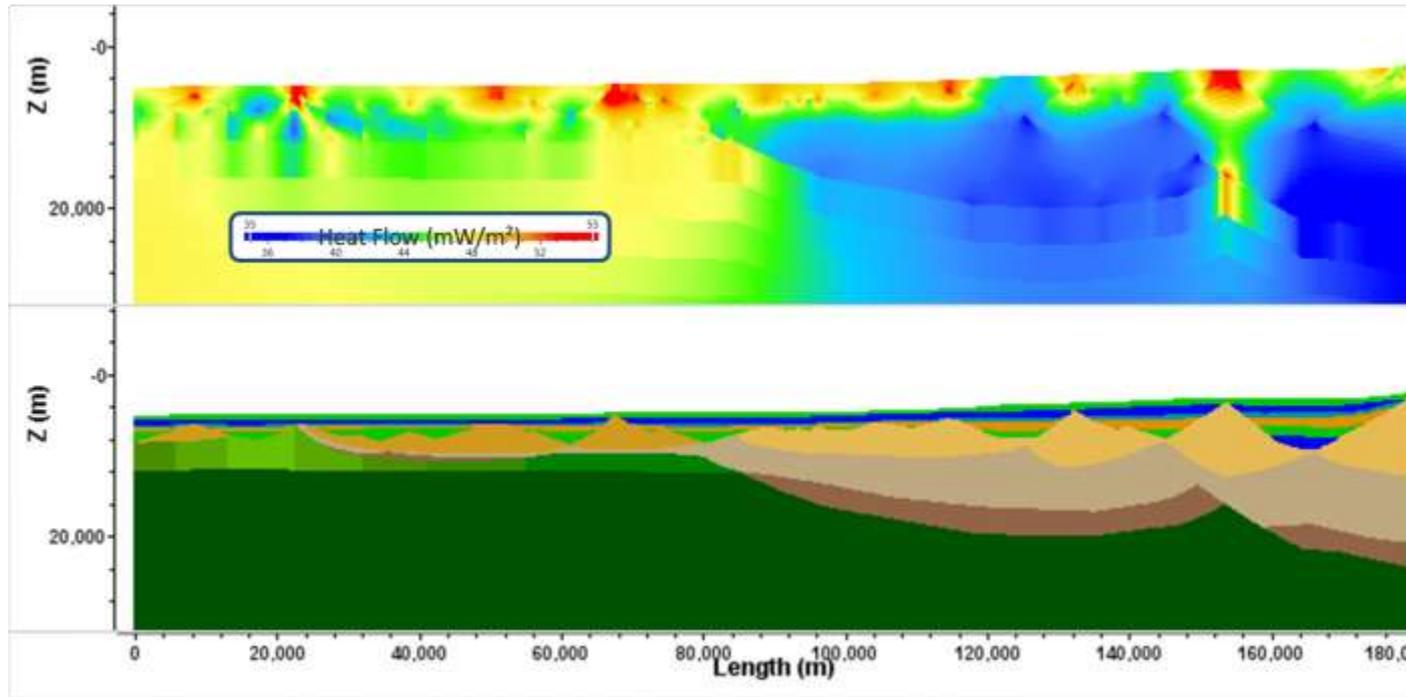
*Coupling of the lithosphere with sedimentation and resulting heat flow distribution. Crust nature and structure have a strong impact on basal heat flow, at present day and through time.*
