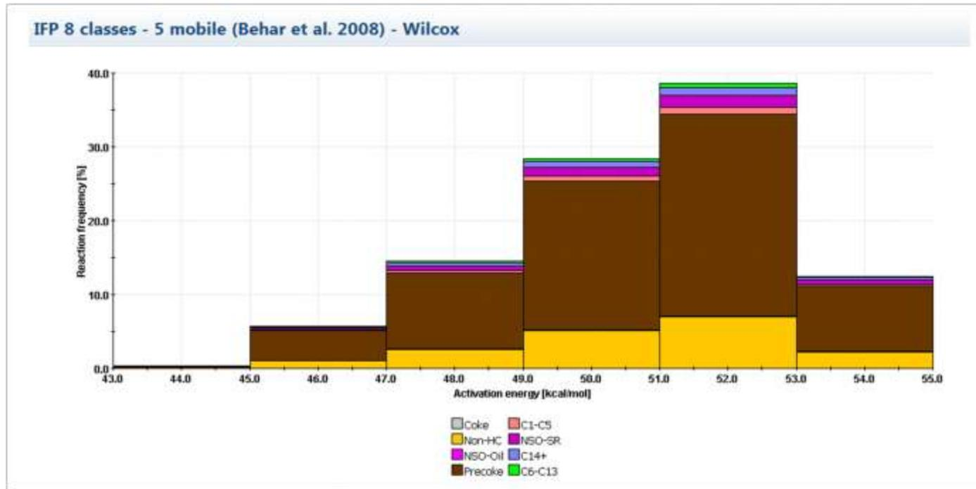
*Thermal cracking of Wilcox kerogen. Extracted from the default IFPEN geochemical library*
