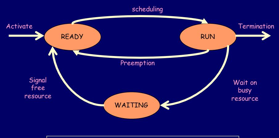
Process/Task state diagram with resource constraints
