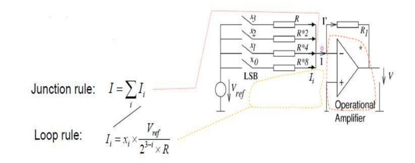
$$I = x_3 \times \frac{V_{ref}}{R} + x_2 \times \frac{V_{ref}}{2 \times R} + x_1 \times \frac{V_{ref}}{4 \times R} + x_0 \times \frac{V_{ref}}{8 \times R} = \frac{V_{ref}}{8 \times R} \times \sum_{i=0}^{3} x_i \times 2^i$$
