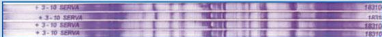
Separation of SERVA IEF Marker Liquid Mix ( pI 3.5 – 10.5) on SERVA IPG BlueStrips pH 3 – 10 (Cat. No. 43012.01, length: 18 cm)
