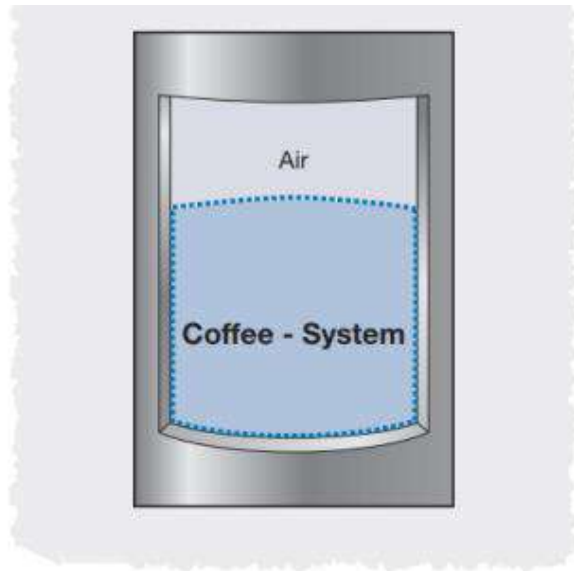
A cutaway diagram of an insulated bottle containing coffee and air, with the system being only the coffee.
